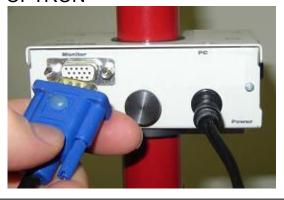
**Step 9:** Plug power supply and monitor cable into a wall socket.
