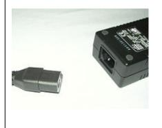
**Step 5**: Connect the power supply cable to the OPTRON
