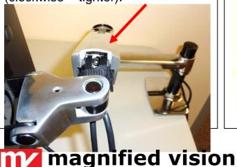
**Step 8:** Squeeze the two lips of the black plastic cover underneath the middle element of the arm and pull the cover away from the base.
