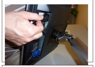
**Step 9:** Insert the two cables from the monitor into the cover. Return the cover into its place.
