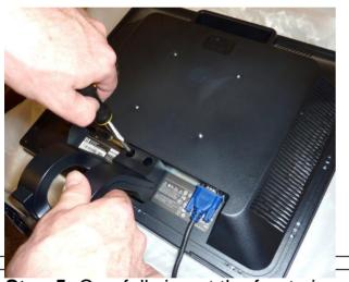
Step 4: Put the monitor on a flat surface (screen facing down) and screw the front piece of the monitor arm to the back of the monitor (thumbscrews enclosed).
