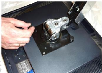
Step 5: Carefully insert the front piece of the arm into the monitor arm extension (or table clamp in the extension is not used).
