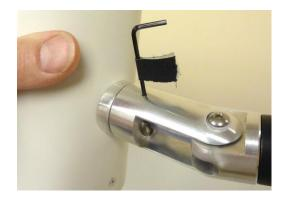
• Tighten or loosen the rotation joint by turning the camera head approximately 5-10 degrees against the blocked bolt. Looking from the steel arm towards the camera head, turn clockwise to loosen or counterclockwise to tighten.
