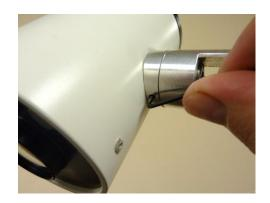
Insert the flagged Allen Wrench into the hole at the top of the joint. Turn the camera head until the Allen wrench sinks a little deeper into the joint and blocks the camera head rotation.
