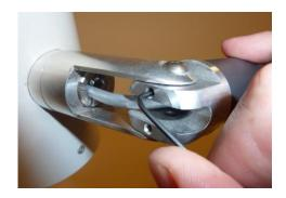
Using the big Allen wrench, tighten or release the joint screw on the top.
