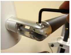
Using the big Allen wrench, tighten or release the joint screw on the bottom.
