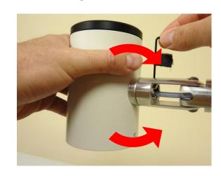
Remove the Allen wrench from the hole and use the same wrench to tighten the set screw. Repeat steps 5-8 if joint wiggles or feels too tight/loose.
